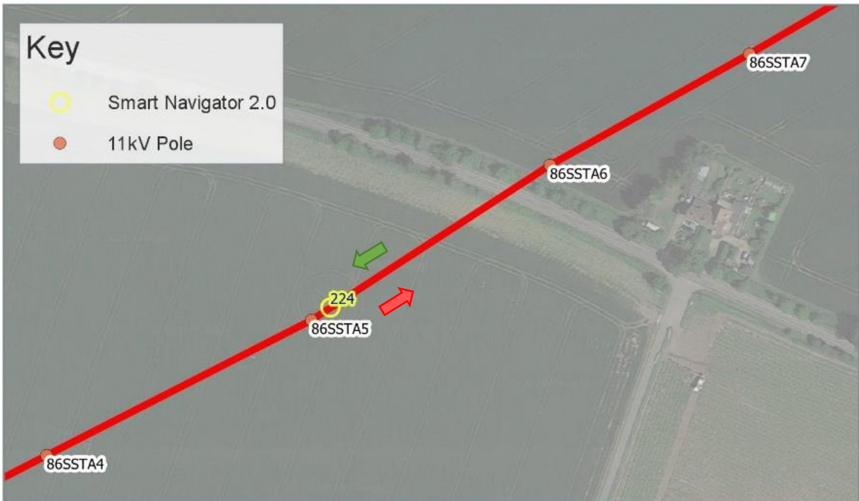
Figure 2-4– Topological view of Site #224 (demonstrating directional power flow convention)
