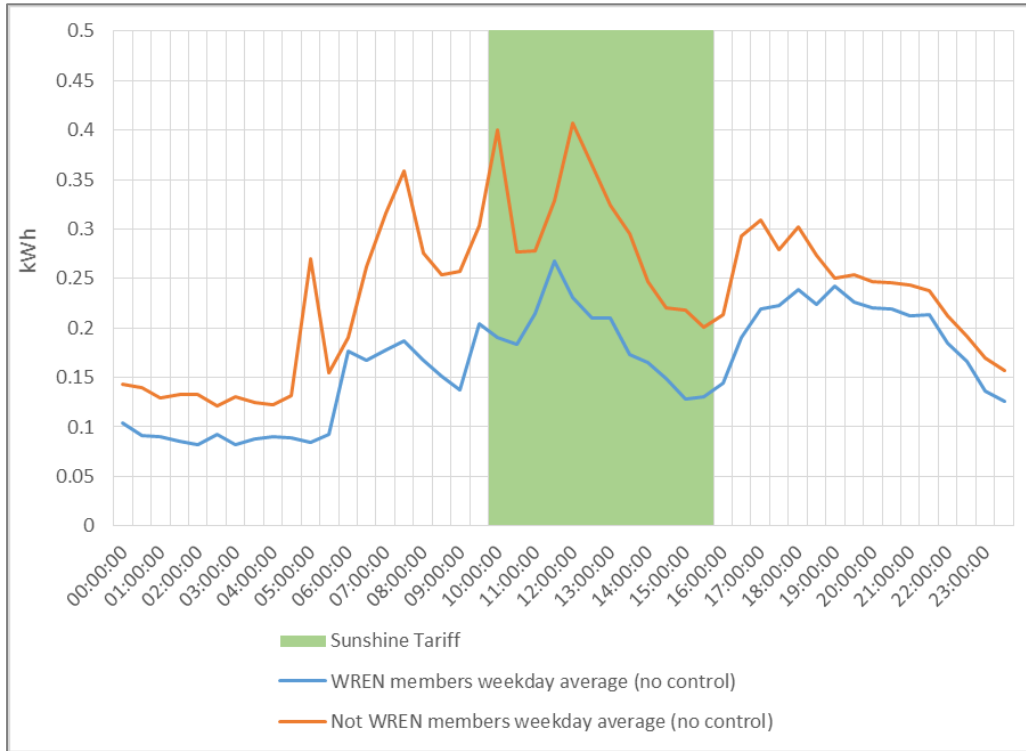
Figure 10 Comparison of demand profile for WREN members and non-members for the average weekday
