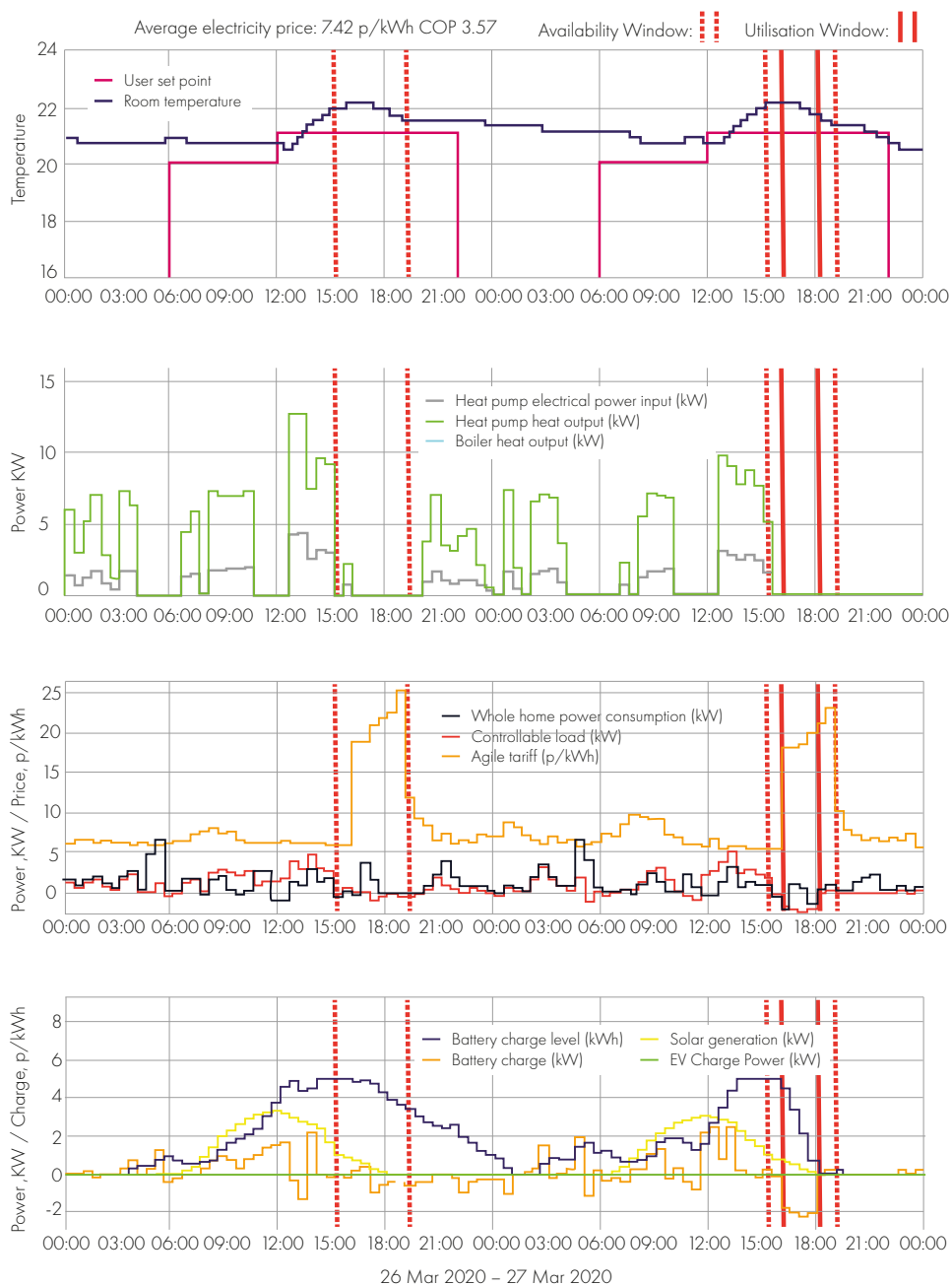
Figure 29 – Dynamic style Flexible Power intervention. This intervention was carried out during Phase 2 of the field trial and thus controllable load refers to heat pump and battery load.
