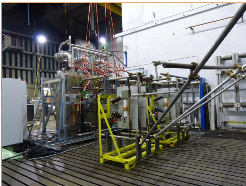
Figure 6-10: Bournville FCL during short circuit testing at the KEMA laboratory
