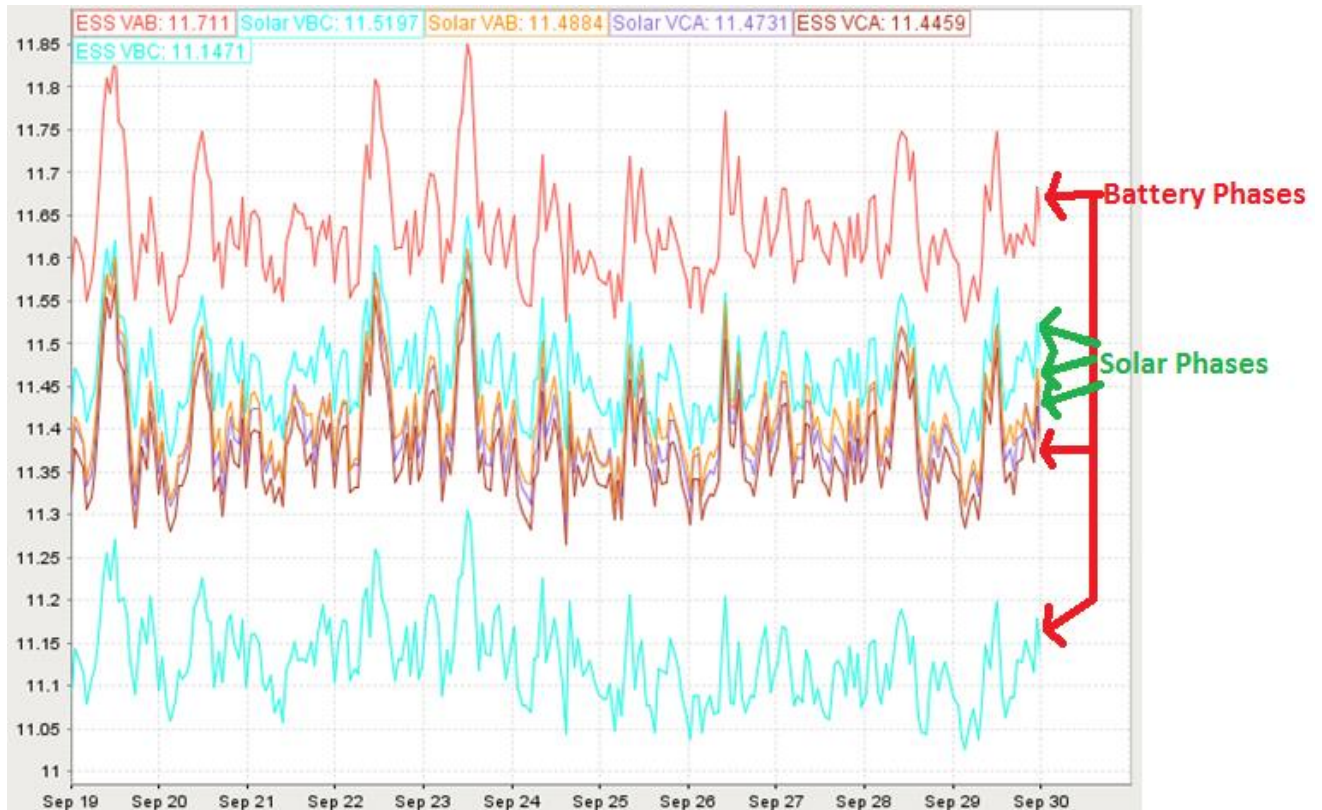
Figure 32: Battery and Solar phase voltages
