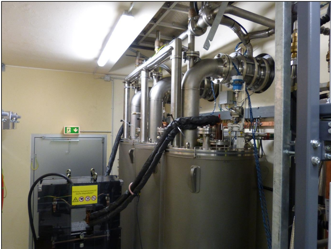
Figure 2-17 - Chester Street FCL undergoing current testing during FAT
