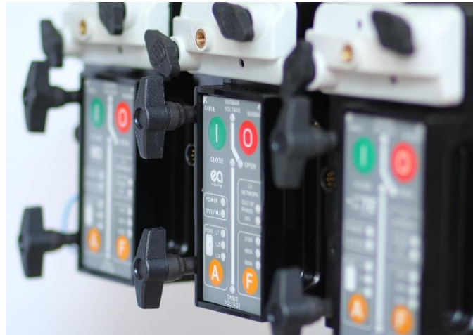
Figure 4: OpenLV Solution – ALVIN Reclose™ devices
