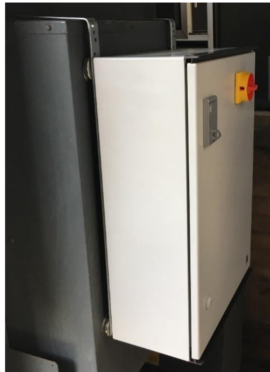
Figure 11: Example of a magnetic mounting
