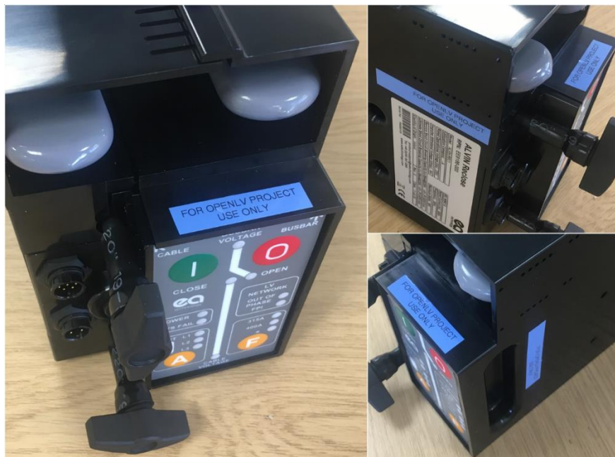
Figure 2 – OpenLV Modified Alvin Reclose™ device
