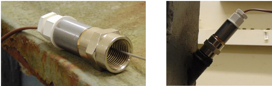
Figure 28: Oil Probe before and after installation
