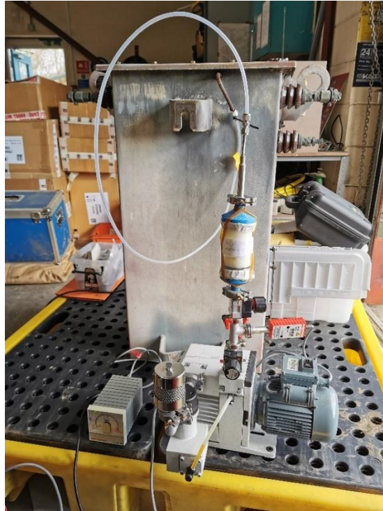
Figure 2.4: Experimental setup using a test transformer with ~50 ppm PCB contamination.
