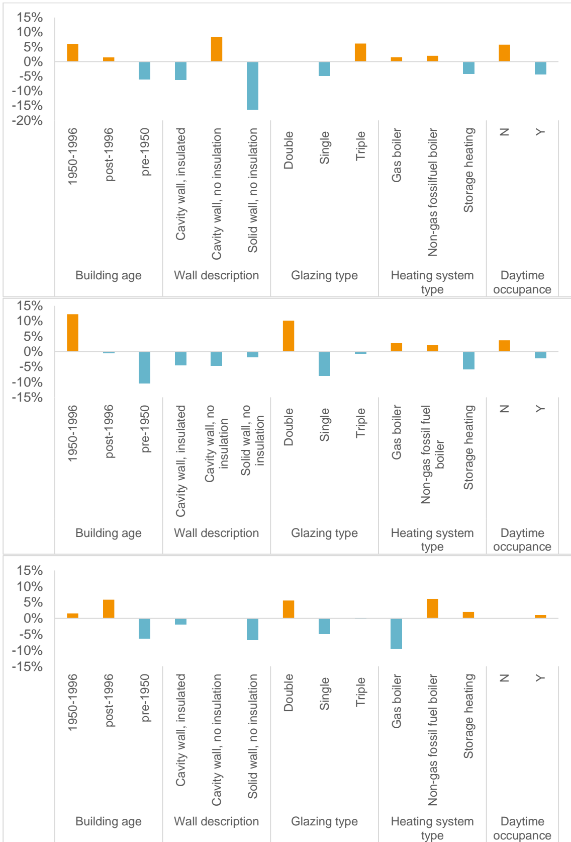
Figure 17 Percentage difference between modelled and actual values in (a) Newport, (b) Mackworth and (c) Bath Road
