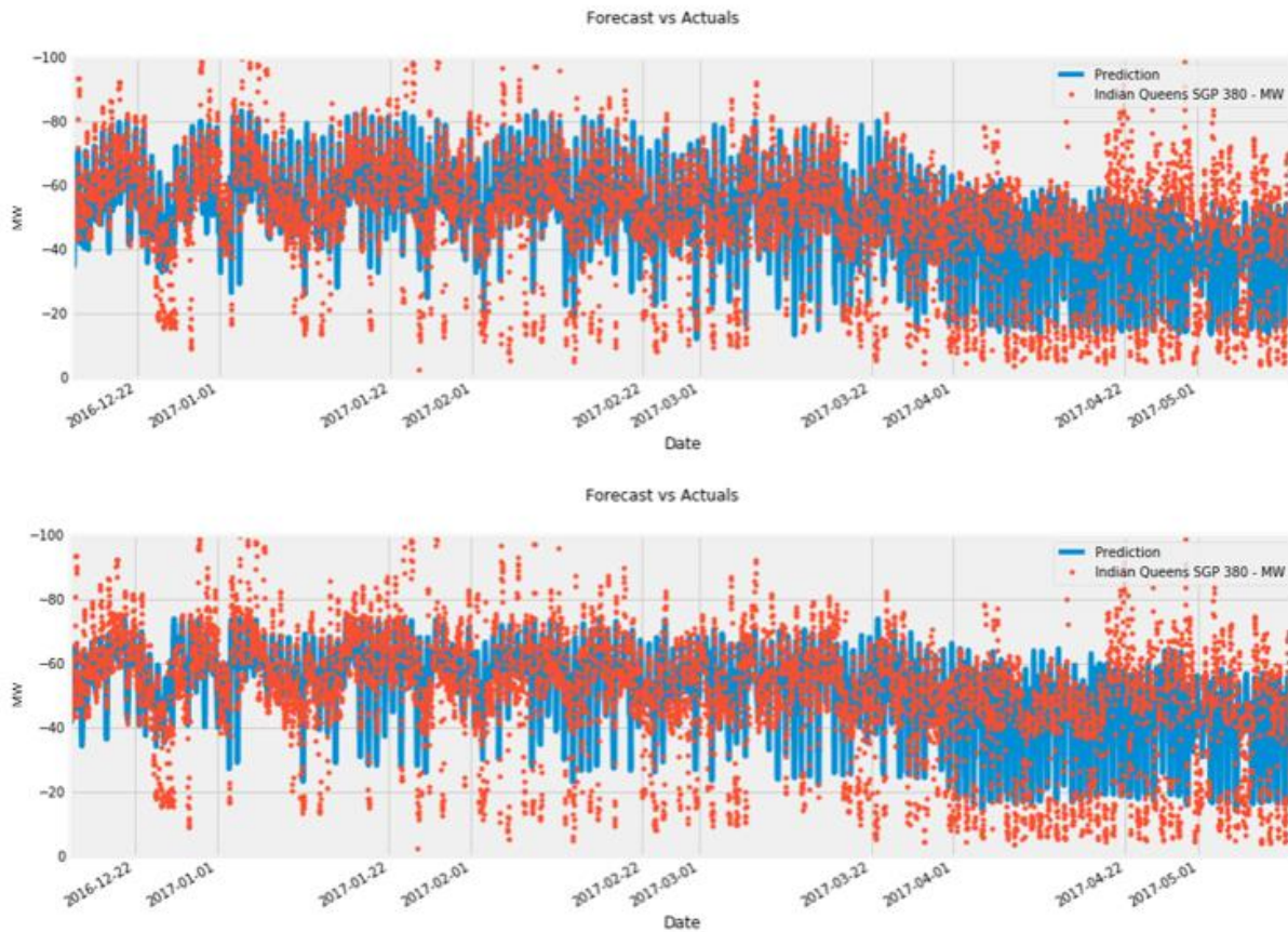
Figure 32: UC1 – Forecast MW versus actual MW data. Top – Forecast 1. Bottom – Forecast 2.
