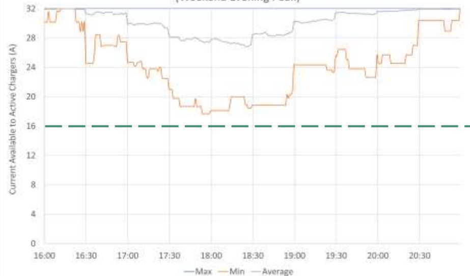
CrowdCharge Trial 1 - Current Available to Active Chargers During Winter (Weekend Evening Peak)
