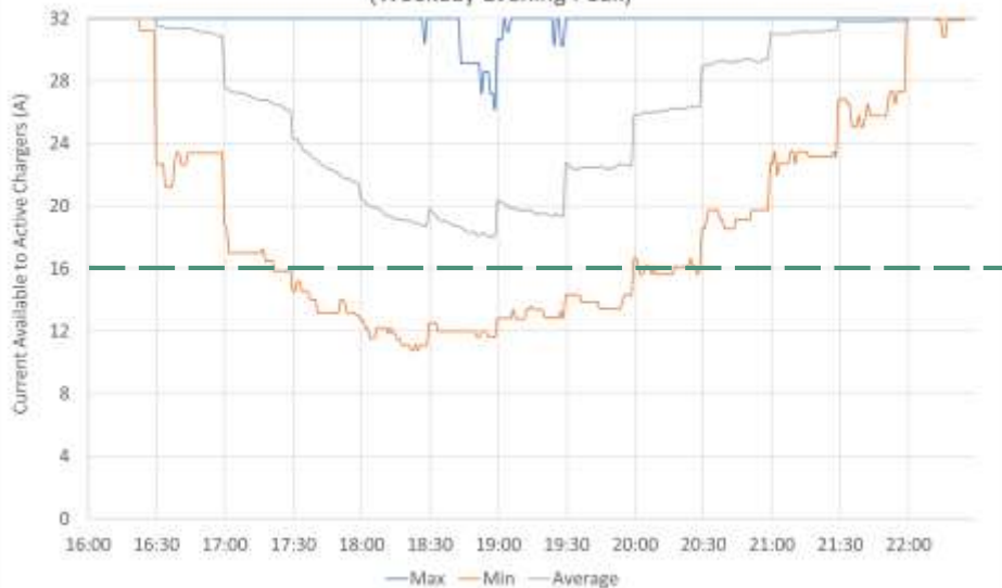
CrowdCharge Trial 1 - Current Available to Active Chargers During Winter (Weekday Evening Peak)
