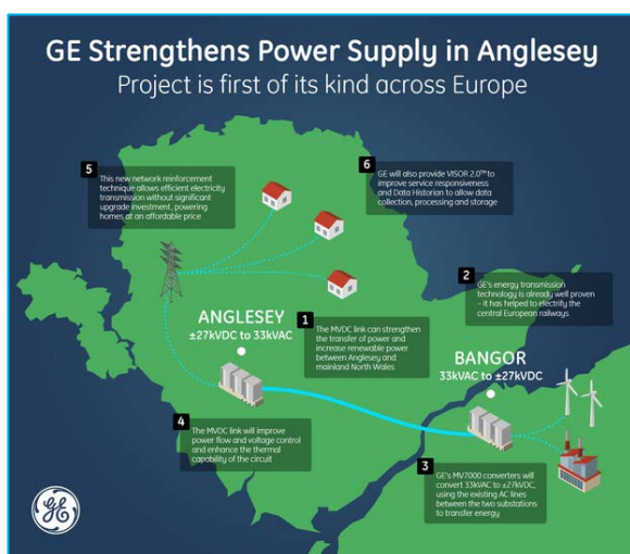
Figure 5-2 – Location of Angle DC MVDC link [4]
