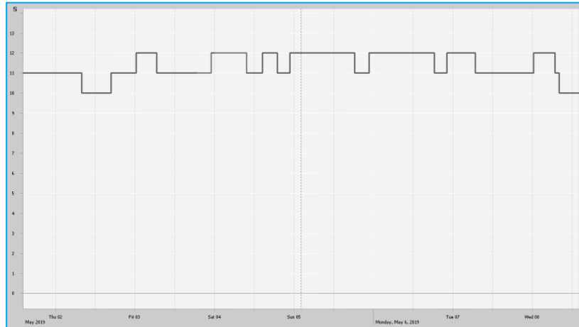
Figure 7-2 – Historic Tap Positions of GT1 at Tiverton BSP during a week in May 2019
