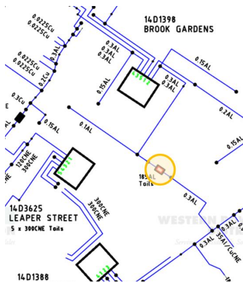
Figure 4: Normally Open Point
