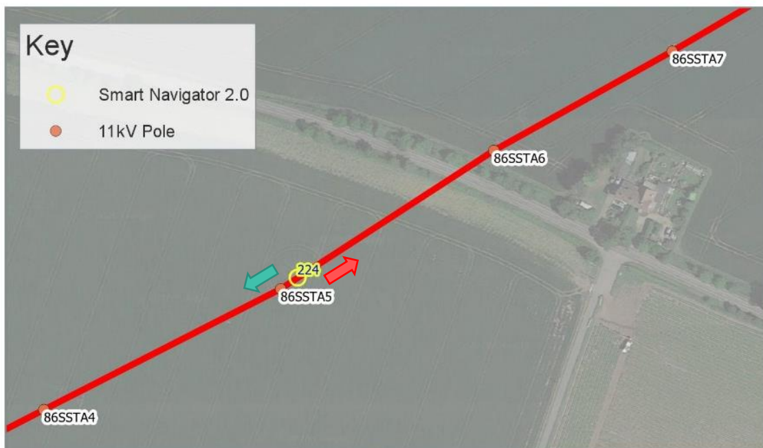
Figure 5-2 –Direction of fault passage through Smart Navigator 2.0 sensors
