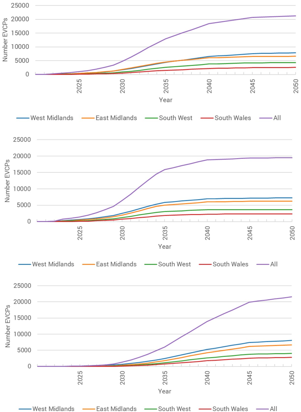
Figure All.4 : Cumulative en route / local charging stations EVCPs deployment across National Grid's Licence areas for Best View (top), Leading the Way (central) and Steady Progress (bottom) scenarios.
