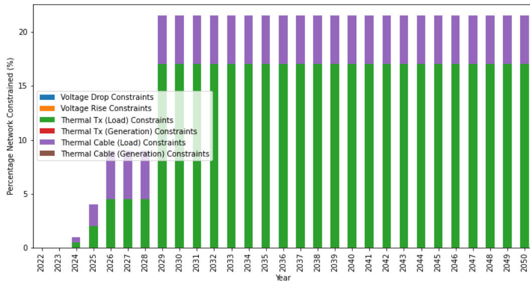
Figure AVIII.11 Cumulative Constraints for network archetype LV11 in South Wales, Best View scenario
