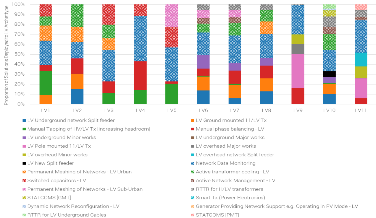
Figure 49: Proportion of BaU and Novel Solutions deployed by LV Network Archetype in East Midlands, Leading the Way scenario
