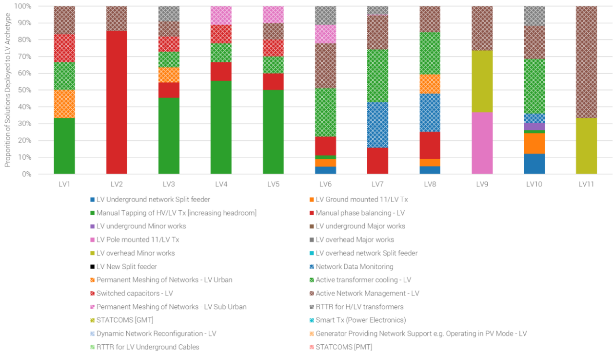
Figure 47: Proportion of BaU and Novel Solutions deployed by LV network archetype in South Wales, Best View scenario
