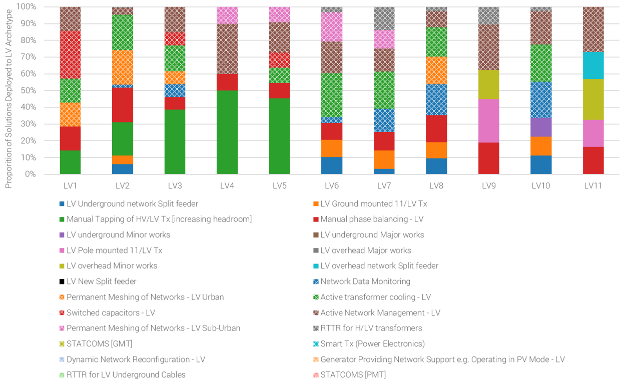
Figure 48: Proportion of BaU and Novel Solutions deployed by LV network archetype in South West, Best View scenario
