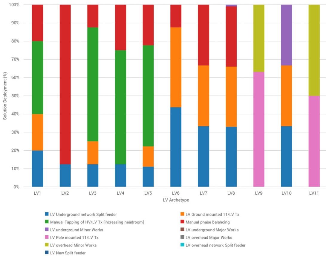
Figure 25: BaU solutions deployed across the LV network archetypes in the Best View scenario in South Wales.
