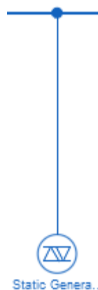
Figure 2 PowerFactory Static Generator
