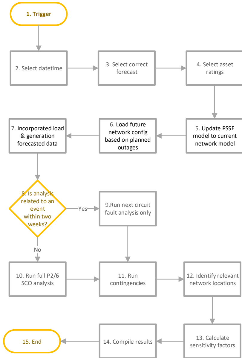
Figure 3: Power system analysis process
