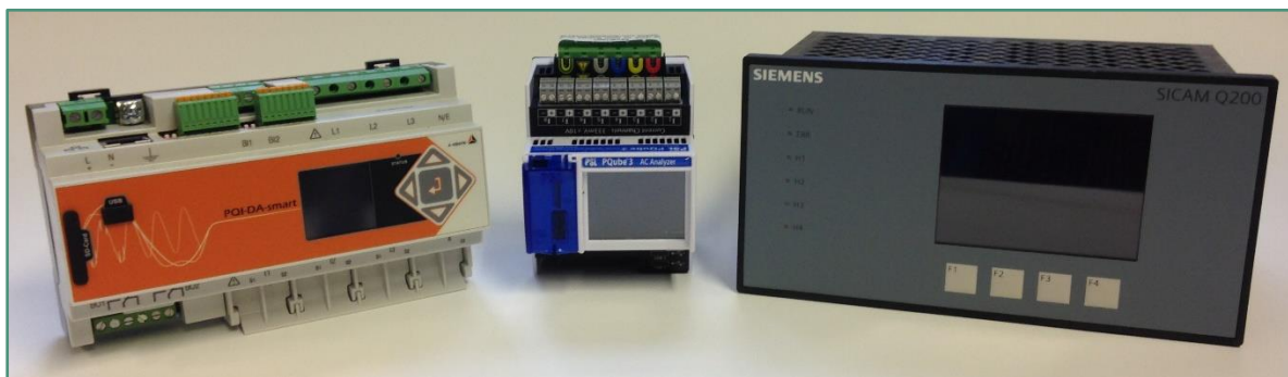
Figure 2-4: The three PQ monitors being used for the project, from left to right: the a-eberle PQI-DA smart, the PSL PQube3, and the Siemens SICAM Q200
