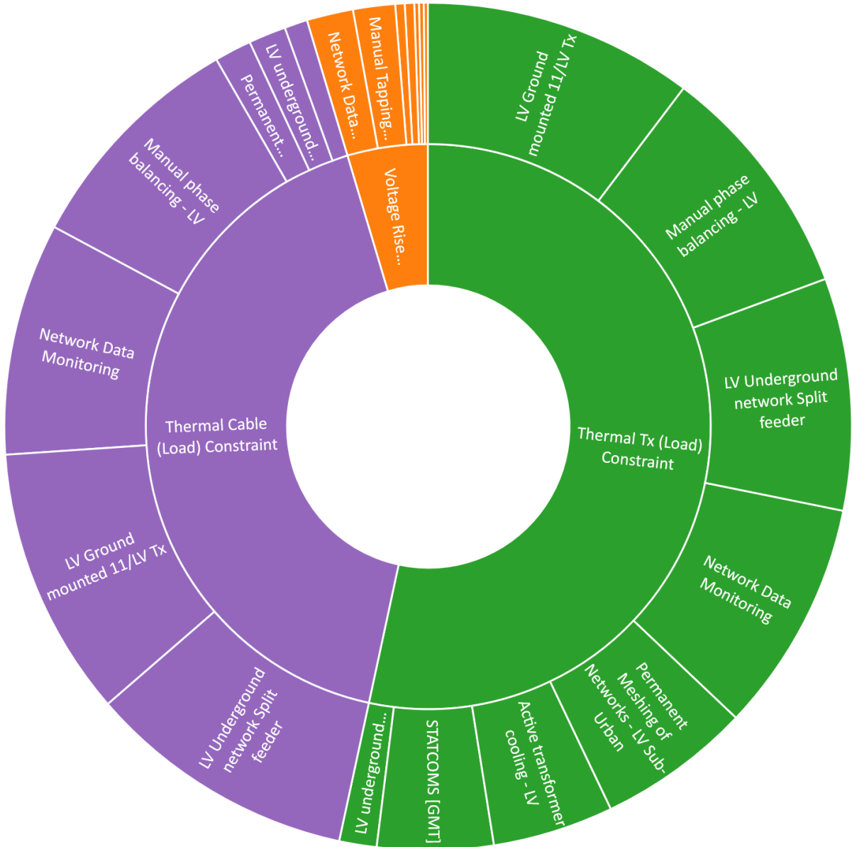
Figure 5: Solutions deployed for constraints on LV2 in East Midlands under BV scenario
