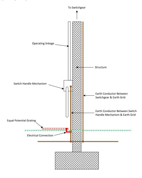
Two connections shall be provided at the grating end of the electrical connection when five gratings are connected together to form a composite grating, one at each end of the "C".
