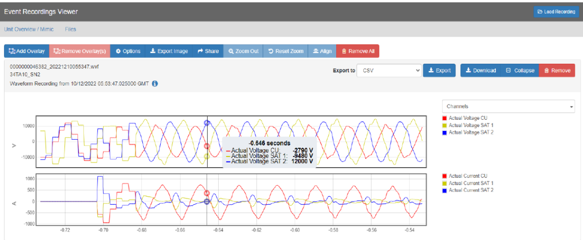
Figure 3 - Class II Device, Smart Navigator 2.0 waveform viewer, including the automatic synchronisation and merging of waveforms
