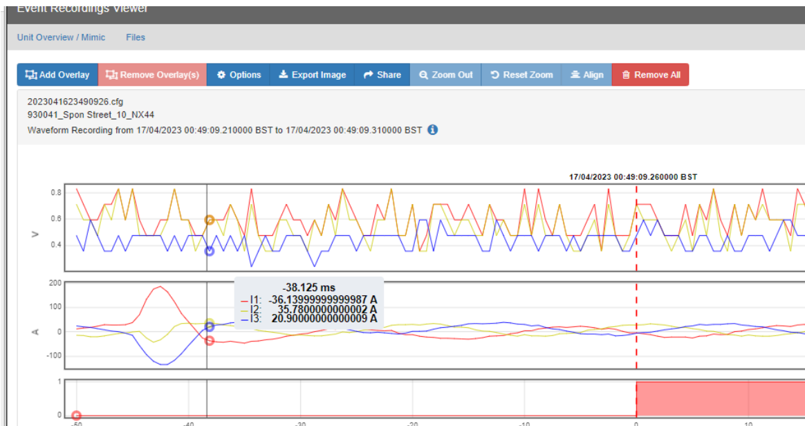
Figure 27 - Example waveform capture due to presence of a genuine network defect
