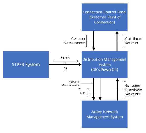
It is expected that the STPFR will be delivered in the same ICCP transfer set as the network measurements. Additionally, the ANM system will have access to a set of static ratings that are used by default if the STPFR is unavailable via the ICCP transfer set.
