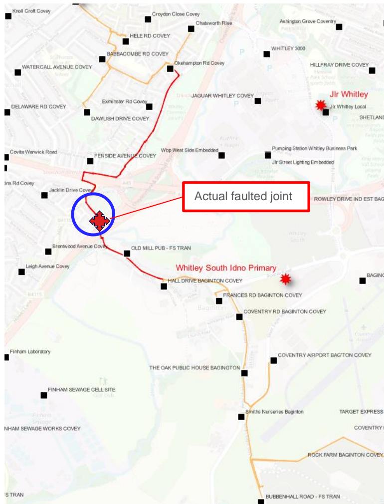
Figure 7.2.9: Fault prediction (blue ring) and actual faulted joint (red indicator) for fault on 10/12/2023.
