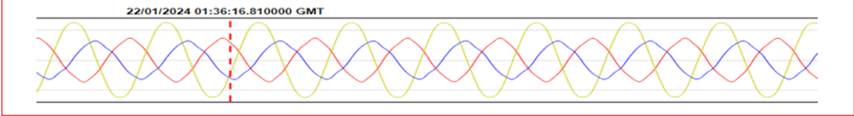
Figure 4.13.2 – Cross-triggering of PQube3 by NX44 to capture a Ph-E fault
