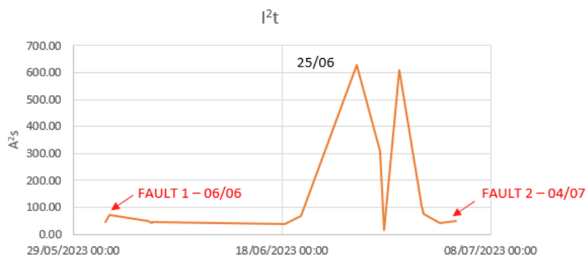
Figure 6.4.9: Time-series plot of the change in I^2t ( A^2s ) showing two large spikes in the pre-fault activity leading up to a post-fault event (FAULT 2).
