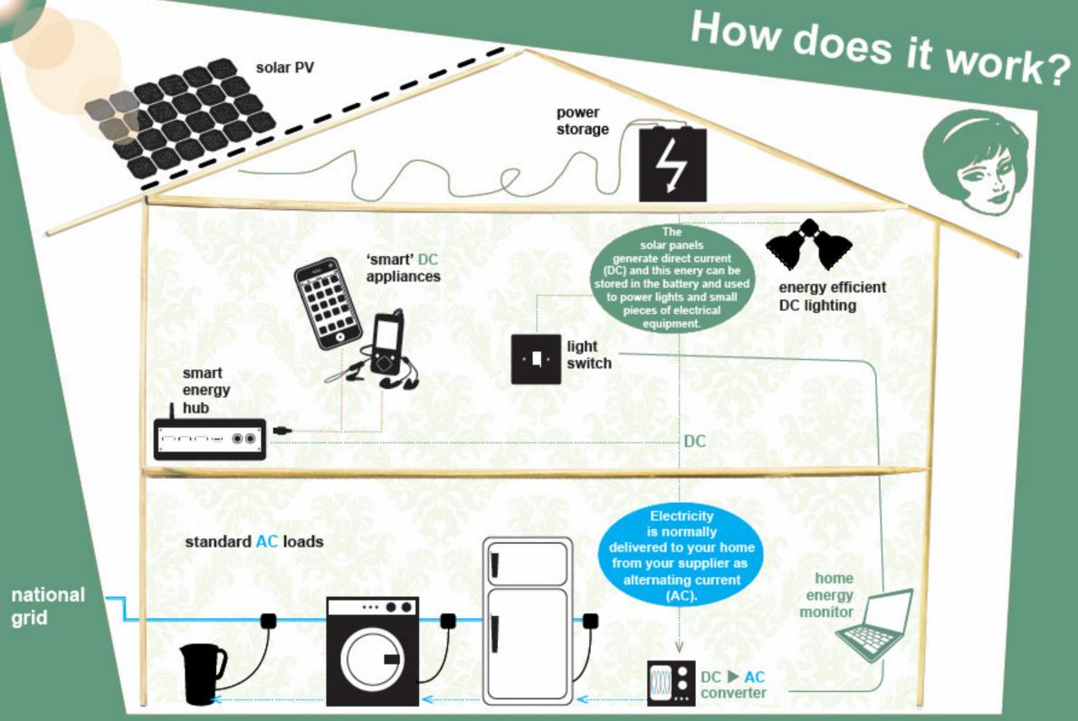
The DC Network and battery will be installed by qualified electricians using the existing lighting circuit within your home. Your house will not need to be rewired. The batteries will either be installed in the loft or outside your house.
